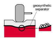
**Filtration:** The geosynthetic acts similar to a sand filter by allowing water to move through the soil while retaining all upstream soil particles. For example, geotextiles are used to prevent soils from migrating into drainage aggregate or pipes while maintaining flow through the system. Geotextiles are also used below rip rap and other armour materials in coastal and river bank protection systems to prevent soil erosion.
