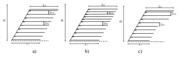
Fig. 2: a) uniform length and uniform spaced reinforcements; b) uniform length reinforcements with reduced spacing at the top; c) uniform spaced reinforcements with increased length at the top.
