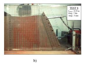
Fig. 3. Response of different reinforced type wall to the same seismic excitation: a) failure of a wall with uniform length and uniform spaced reinforcements; b) acceptable permanent displacement of a wall with uniform length and reduced spacing of reinforcements in the upper part of the wall.
