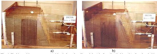
Fig. 1 Shaking table test on a geogrid-reinforced wall model: a) before the shaking; b) after the shaking
